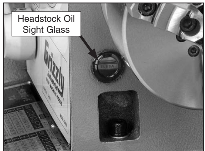
Figure 12. Headstock oil sight location.
